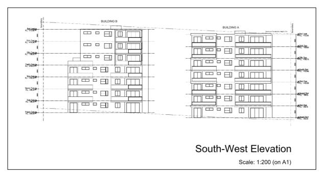
As shown on the Section drawing above the majority of the development is below the height limit, with the exception of the lift overruns which protrude above the height plane by up to 600mm or 2.86%.
